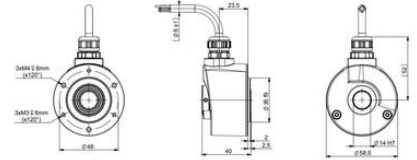
AH05S14/DM/ Flange side clamping, Connection BFR (Radial M12)
