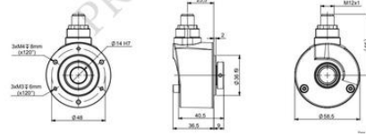
DH05S14/OM Flange side clamping, Connection GMR (Radial M12)
