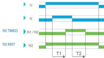
Function Ac - On/Off Delay (Delay on make/break)
