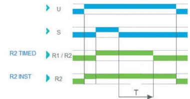
Function C - Off-Delay (Delay on break)
