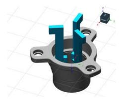
The main application (R3DVi Runtime), takes care of locating the objects and communicating with the robot (or other device). It has a touch-screen friendly graphical user interface that includes 3D visualization of the scanned scene and located objects. A one-time calibration procedure allows the results to be given in the desired robot coordinate system.
